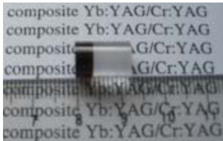
Fig. 1 Photograph of composite Yb:YAG/Cr:YAG ceramics ( \phi 8 \times 12 mm), the thickness of Yb:YAG and Cr:YAG are 8 mm and 4 mm, respectively.
