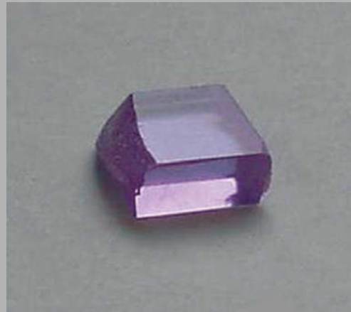
Sample of (La 1-x Nd x )BO 2 MoO 4 prepared from a crystal grown from the melt
