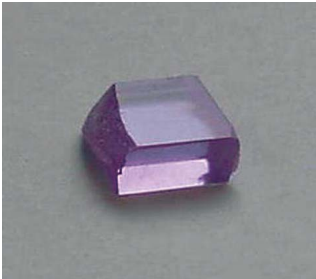
Figure 4 (online color at www.lphys.org ) Sample of (\text{La}_{1-x}\text{Nd}_x)\text{BO}_2\text{MoO}_4 with x \approx 0.047 , prepared from a crystal grown from the melt. Size of sample 6.0 \times 5.8 \times 2.4 \text{ mm}^3
