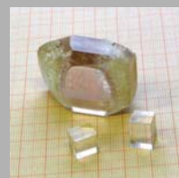
Example of a grown crystal of \text{PbB}_4\text{O}_7 , together with two crystal samples that were cut from the bulk of the crystal
