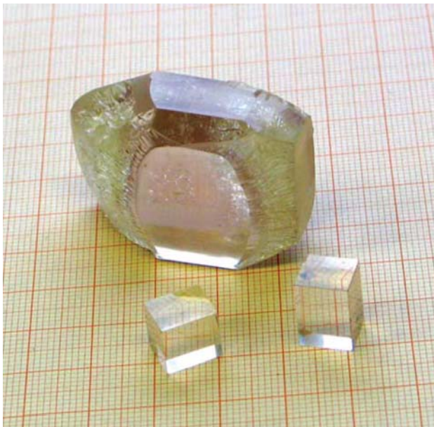
Figure 2 (online color at www.lphys.org ) Example of a grown crystal of \text{PbB}_4\text{O}_7 , together with two crystal samples that were cut from the bulk of the crystal
