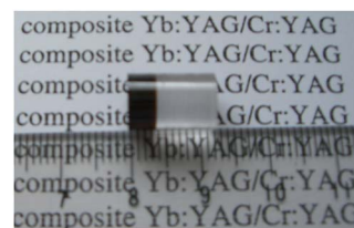
FIG. 1. (Color online) Photograph of composite Yb:YAG/Cr:YAG ceramics ( \phi 8 \times 12 mm); the thickness of Yb:YAG and Cr:YAG are 8 and 4 mm, respectively.
