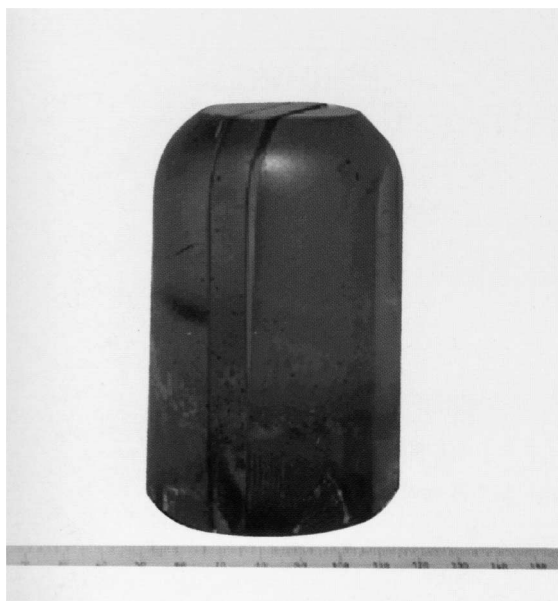
Fig. 1. Highly doped Nd:YAG crystal grown by TGT ( \phi 60 \times 100 mm).
